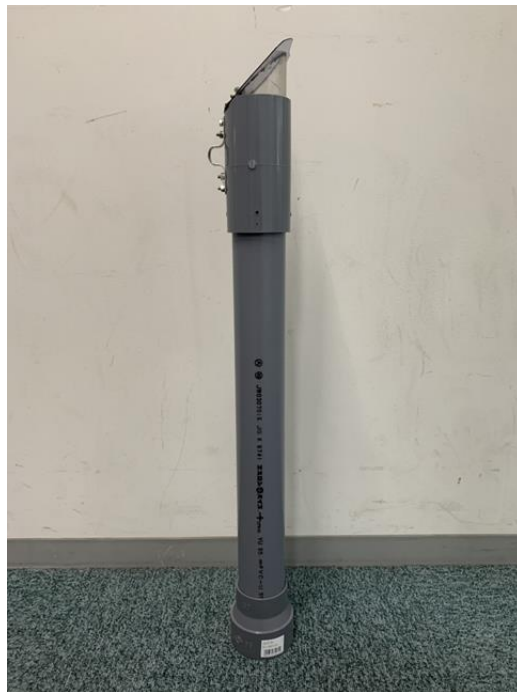
Fig.5 Wave-powered upwelling pump
