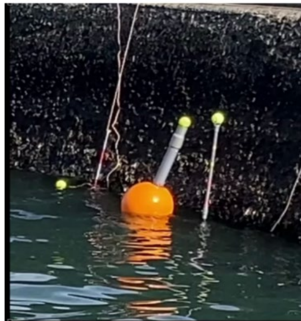
Figure 15 Upwelling pump by wave energy State of installation
