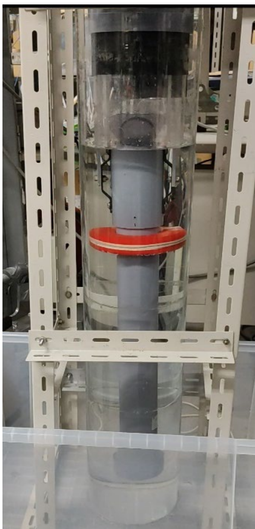
Figure 48 Wave upwelling pump (Statically determinate state)
