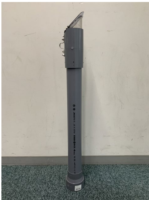
Figure 46 Upwelling pump by wave energy
