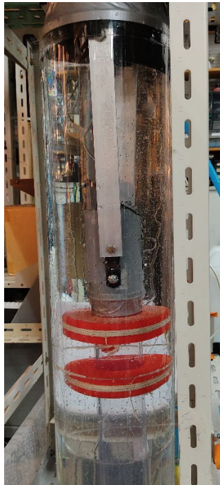
Figure 58 Upwelling pump in lower water tank
