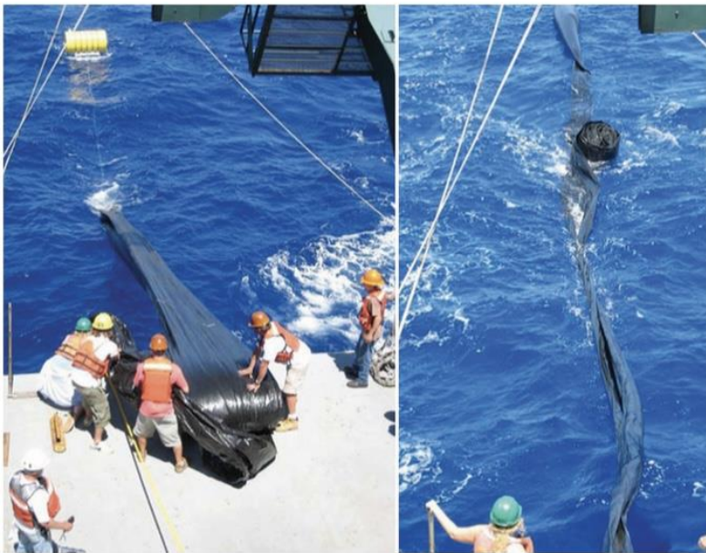
FIG. 3. Image of the deployment of the single pump. With the ship moving forward at 2 kt, the buoy of the single pump was deployed. The main masses of the pumps were then deployed with the bottom valve of the pump system secured on deck. The forward motion of the ship causes the tube to slowly unwind to achieve full length. After it was fully opened, the valve and recovery line were deployed.
