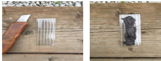
Silicone coated polycarbonate for repair
